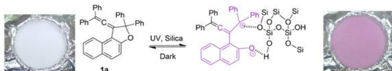
Scheme 2: Photochromic equilibrium for new 1-vinylidene-naphthofuran 1a (Ar=Ph) and photographs of silica gel doped with this compound before and after UV irradiation (365 nm)
